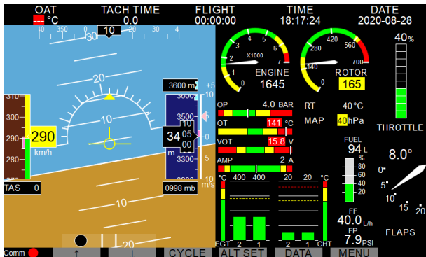
Engine parameters & flight attitude integrated screen (closed automatically when attitude module is off)
