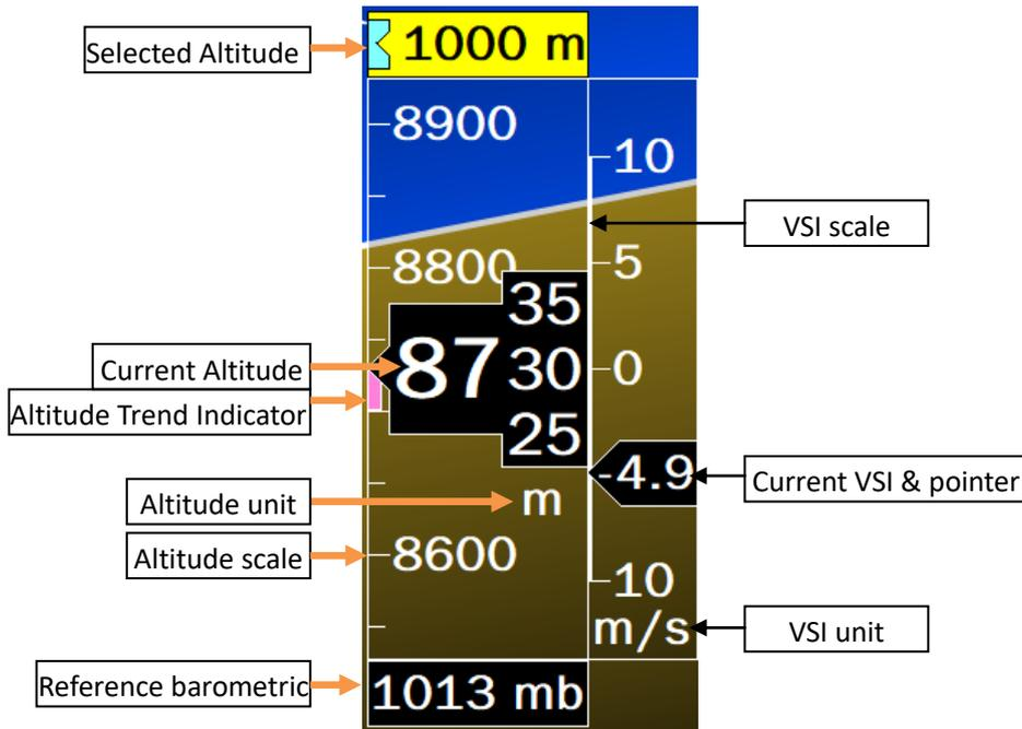
Fig. 26 Altimeter, vertical speed indicator and reference barometric
