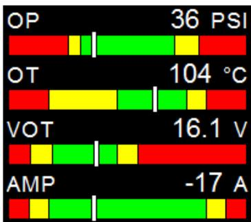
Fig. 18 Oil pressure, oil/water temp, voltage, current indicator
