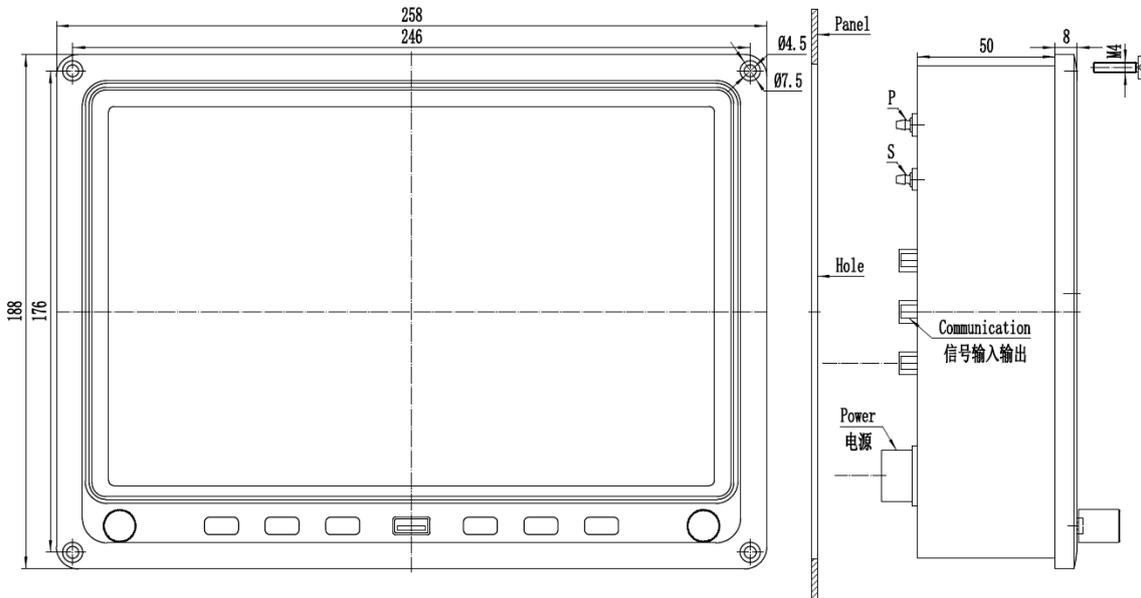
Fig. 2 Product outline and dimensions (in millimeters)
