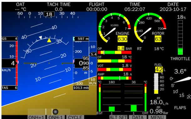
Engine parameters & flight attitude integrated screen (Not automatically when attitude module is off)
