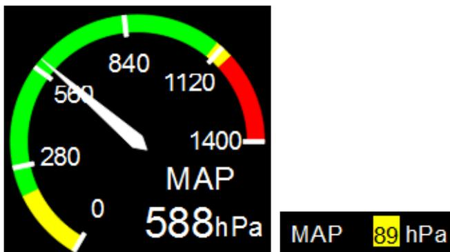
Fig. 12 Manifold pressure indicator
