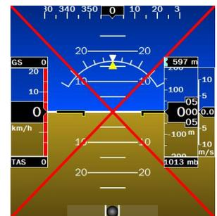
Fig. 29 AHRS not connected
