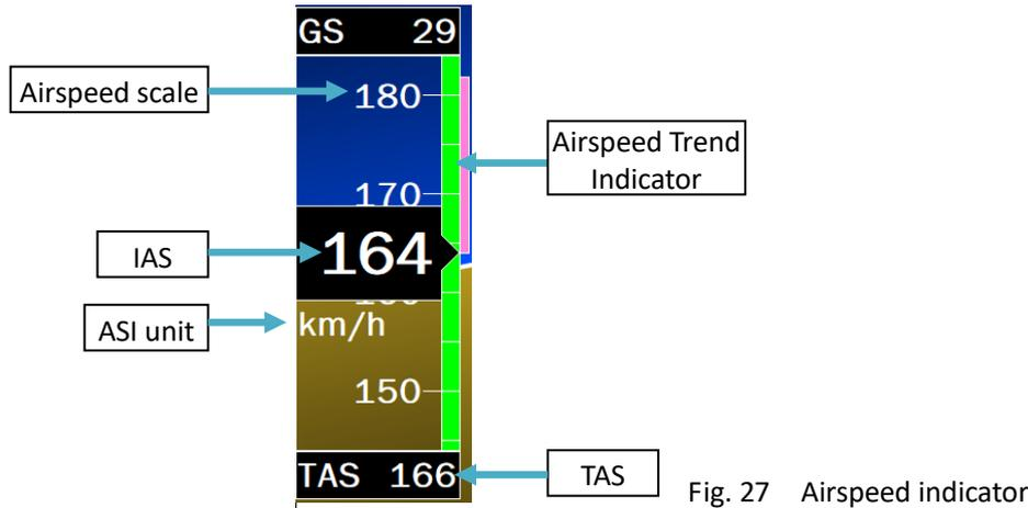
Fig. 27 Airspeed indicator
